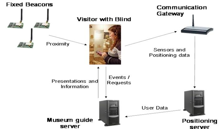
Figure 1 – PIL system architecture
